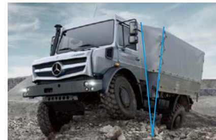
Diagonal torsional flexibility with torque tube technology
