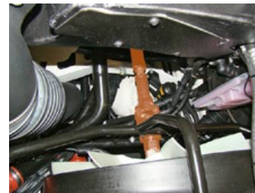
Fan with electronic viscous clutch, mechanically driven via propeller shaft
