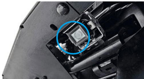
Front camera under bumper
