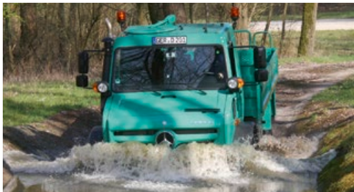
Standard fording capability to 80 cm
