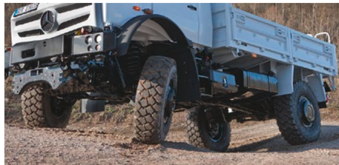
3-point mounting of engine, gearbox and cab. Double 3-point body mounting
