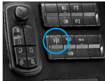
Transmission PTO switch
