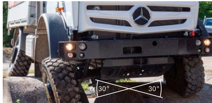
Major axle articulation made possible by torque tube concept and coil springs
