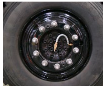
Left: attachable hose line, test and filling valve for rim and tyre
