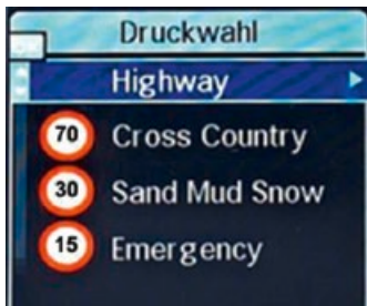
Pre-selection of tyre pressure on display, operation via steering wheel buttons
