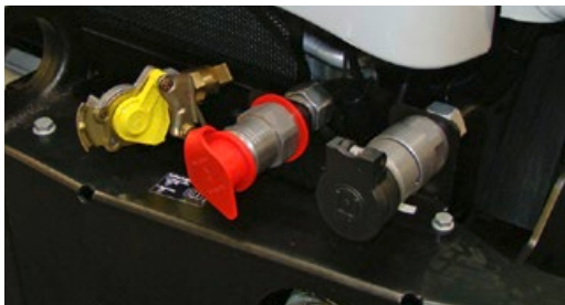
Hydraulic system [H10]: Plug connections at front on the left in direction of travel: delivery line (red) and return line (black)
