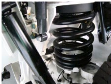
Coil springs with telescopic shock absorbers
