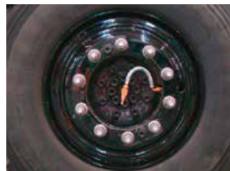
Left: air supply to the valve (no wheel cover)
