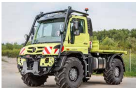
Vehicle with [VT1] – Registration as tractor, Europe, [FP4] – Pre-installation of cab roll cage and [UFPK] – Cab roll cage
