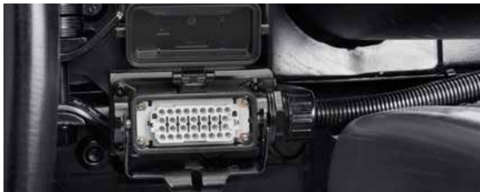
[E87] – Equipment socket, 32-pin
