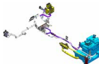
Hydraulic system, single-circuit, 2-cell, fully proportional [HN2]
