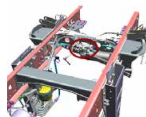
UGE with ALB controller (configuration for U 200)
