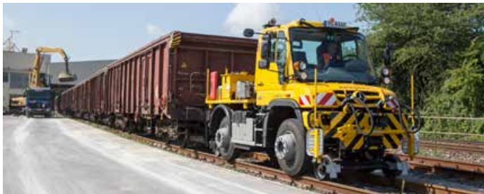
Road/rail use with torque converter clutch
