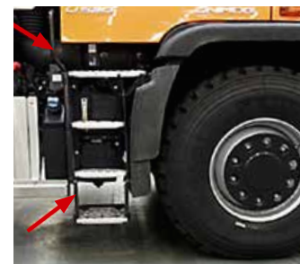
4-step access on right, in accordance with tractor standard
