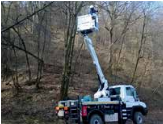
Operation of elevating work platform via power take-off
