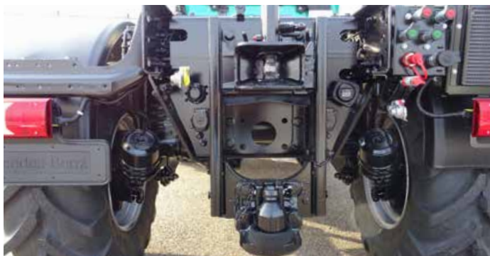
[Q34] – End crossmember, reinforced, for lowered trailer coupling [UQSL] – Bearing bracket for Scharmüller height-adjustable trailer coupling [UQSM] – Trailer coupling, Scharmüller, pin 38 [UQSN] – Trailer ball coupling K80, Scharmüller
