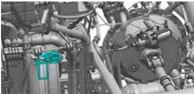
Socket, 11-pin, behind cab on left [ES6]
