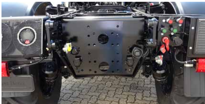
[Q34] – End crossmember, reinforced, for lowered trailer coupling
