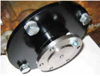
[N13] – Transmission PTO, high speed, with 6 hole flange
