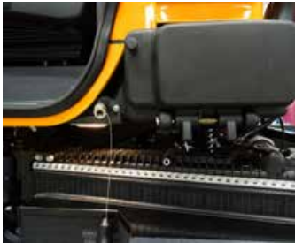
[L60] – Entrance lights in step area, incl. compressed-air connection
