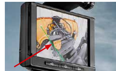
Green guide lines on the monitor display to assist with implement mounting
