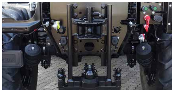
[Q34] – End crossmember, reinforced, for lowered trailer coupling [UQSK] – Bearing bracket, for height adjustable trailer coupling, incl. K80 [UQSM] – Trailer coupling, Scharmüller, pin 38 [UQSZ] – Articulated steering K50, left and right, for 3 t drawbar load
