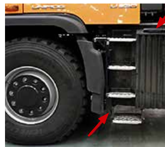
4-step access on left, in accordance with tractor standard
