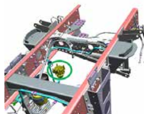
UGE without ALB controller with relay valve (configuration for U 300 to U 500)
