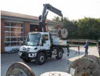
Crane operation via power take-off
