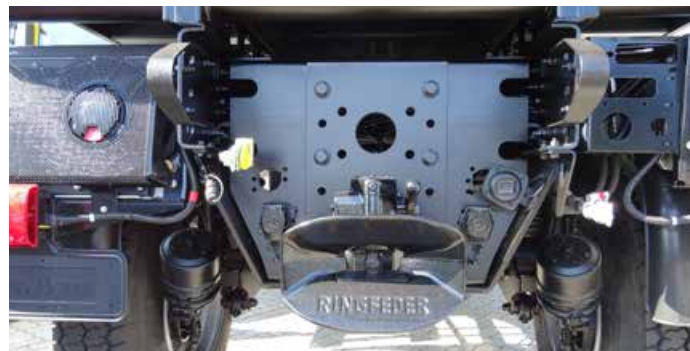
[Q34] – End crossmember, reinforced, for lowered trailer coupling [Q94] – Trailer coupling, large jaw, Ringfeder, pin 38.5
