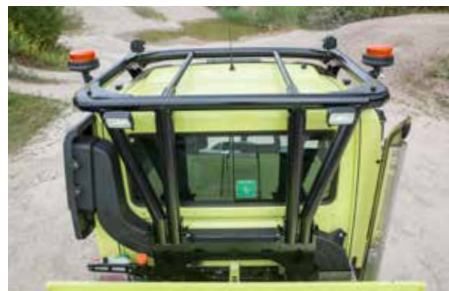
Vehicle with [VT1] – Registration as tractor, Europe, [FP4] – Pre-installation of cab roll cage and [UFPK] – Cab roll cage
