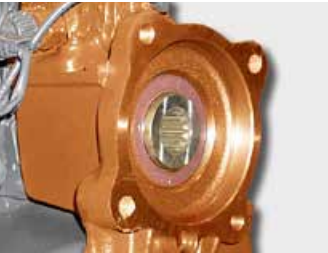
[N16] – Transmission PTO, high speed, with 4-hole connection
